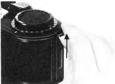
1) Turn the Open/Close Knobs on the top of each magazine to "OPEN" and release the back cover of the 250 Film Back by lifting on the Rear Cover Lock Key. Remove the cover by shifting it slightly to the left and lifting off.
