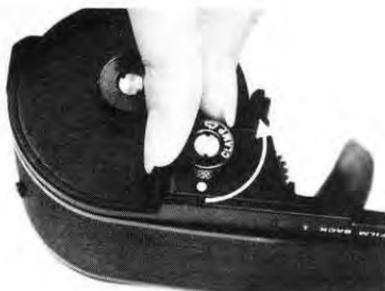
3) Turn the Camera Clamp Knob at the base of the right Magazine Chamber in the opposite direction of the arrow until it stops. This will release the Camera Clamp Plate and allow you to attach the Film Back to the OM-1.
