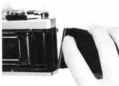
1) Remove the standard back of the OM-1 by opening the cover fully and pressing down on the Rear Cover Release Pin.
