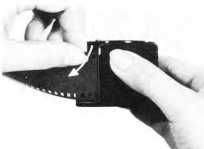
3) Remove the left film magazine, and cut the film by pressing it against the film cutter of the take-up magazine and tearing towards you and down. This leaves a leader extending from the left magazine to be used for spooling the remaining unexposed film.
