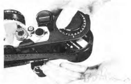
2) Turn the Open/Close Knobs on both chambers to "OPEN". Pull up on the rear Cover Lock Key and remove the rear cover.
