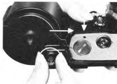
5) While pressing the right side of the camera against the Film Back, turn the Camera Clamp Knob in the direction of the arrow until it stops. The Camera Clamp Plate will close locking the camera firmly against the Film Back 1.
