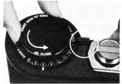
9) Turn the Open/Close Knob on top of the left chamber to "CLOSE". This extends the Camera Holder and opens the Supply Magazine.
