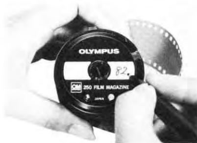
4) To remove the right magazine, pull down on the Fork Knob of the right chamber and remove the magazine by inverting the Film Back and shaking gently.
