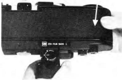
7) Place the rear cover of the 250 Film Back on by hooking the left end onto the catch provided at the left end of the Back. Carefully press the right end into place so the hooks of the cover slide under the edge of the back and snap into place.
