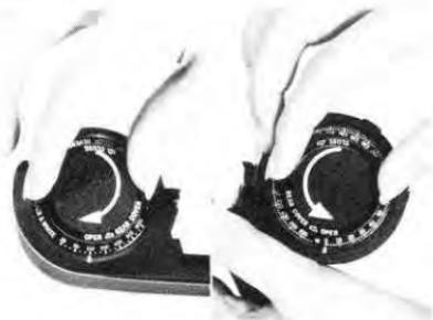
2) Turn the Open/Close knob on top of each Magazine Chamber on the Film Back toward the "REAR COVER OPEN" position until it stops.
