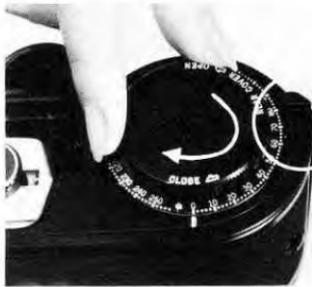
8) Turn the Open/Close Knob on the right chamber to "CLOSE". This locks the Camera Clamp Knob and Rear Cover Lock Key into place, and opens the Take-up Magazine.
