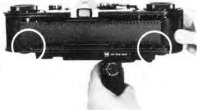
3) Place the supply magazine in the left chamber and the take-up magazine in the right. Line up the red index marks on the magazines with the white index marks on each chamber and snap the magazines into place.
