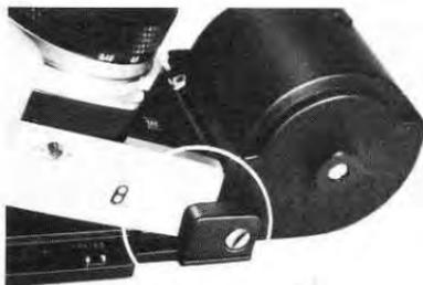
4) Place the left side of the camera (side with Rewind Crank) on the Camera Stage of the Film Back and push the camera towards the Back until the two units are flush against each other.
