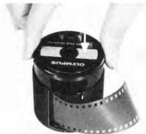
3) Continue spooling the bulk film with the emulsion side down until the desired length has been reached. Cut the film end from the bulk film roll.
