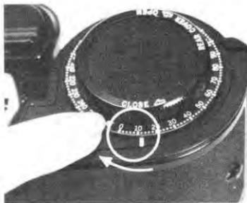
1) When the motor drive stops and the Exposure Counter indicates the last frame has been exposed ("0"), turn the Exposure Counter back to 10 frames ("10"). Cover the camera lens and advance the film 6 frames. This will safely wind the last few exposed frames into the take-up magazine to prevent fogging when opening the back.
